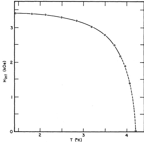
FIG. 3. Experimental  $(H, T)$  phase diagram for  $\text{Ni}(\text{NO}_3)_2 \cdot 2\text{H}_2\text{O}$  with  $\mathbf{H} \parallel a$  axis.
