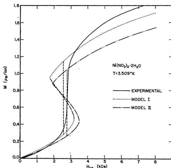
Fig. 6. Comparison of observed and calculated isotherms at 3.51°K for  $\text{Ni}(\text{NO}_3)_2 \cdot 2\text{H}_2\text{O}$  with  $\mathbf{H} \parallel a$  axis. Models I and II are described in the text.
