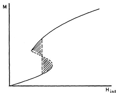
Fig. 4. Schematic magnetization isotherm for two sublattice metamagnet at  $T$  less than but near  $T_c$ .
