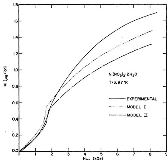
Fig. 5. Comparison of observed and calculated isotherms at 3.97°K for  $\text{Ni}(\text{NO}_3)_2 \cdot 2\text{H}_2\text{O}$  with  $\mathbf{H} \parallel a$  axis. Models I and II are described in the text.
