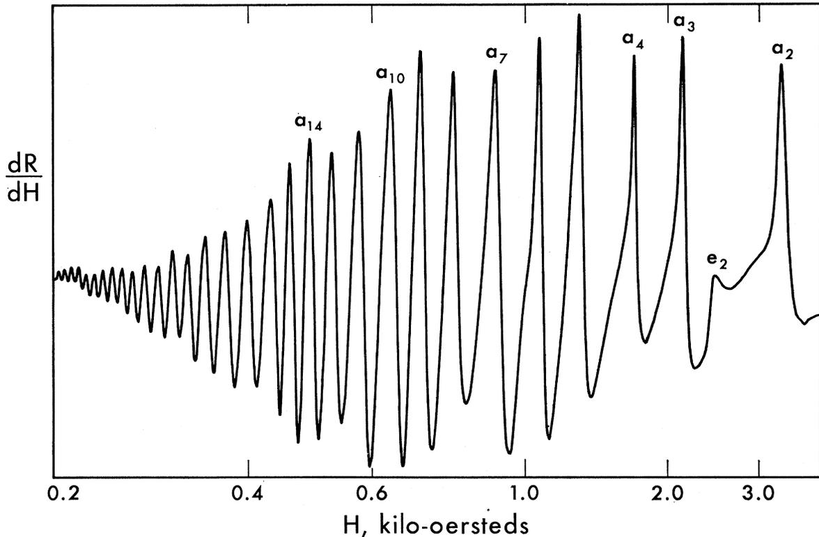
FIG. 4. Cyclotron-resonance signals in zinc for  $\mathbf{H}$  parallel to  $(11\bar{2}0)$  in a  $(10\bar{1}0)$  surface with  $\mathbf{E}_{rf}$  perpendicular to  $\mathbf{H}$ . The magnetic field scale is linear between each field value.
