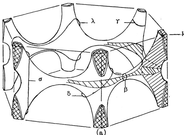
FIG. 2. Fermi surface of zinc according to Gibbons and Falicov. (a) First and second bands of holes (first-band "caps" are shown cross hatched). (b) Third band of electrons.
