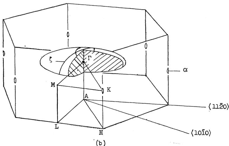
tron surfaces. One forms a surface, the lens, centered at the point  $\Gamma$ , and the other is an elongated ellipsoid structure, the needle, centered at the point  $K$  of the Brillouin zone. The Greek letters in Fig. 2 indicate orbits on the Fermi surface which are referred to in the following discussion.
