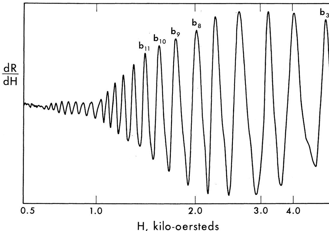
FIG. 5. Cyclotron-resonance signals in zinc for  $\mathbf{H}$  parallel to  $\langle 0001 \rangle$  in a  $(10\bar{1}0)$  surface with  $\mathbf{E}_{rf}$  parallel to  $\mathbf{H}$ . The magnetic field scale is linear between each field value.
