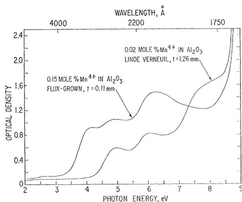
FIG. 8. Absorption spectrum of two different samples of  $\text{Mn}^{4+}$  in  $\text{Al}_2\text{O}_3$ . All bands, except the very weak ones between 2 and 3 eV, are due to charge transfer. The peak near 4.1 eV for the flux-grown sample is believed to be the  $\text{Mn}^{3+}$  charge-transfer threshold.
