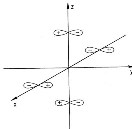
FIG. 4. Electron distribution for the  $t_{2u}(\pi)$  nonbonding molecular orbital. This is believed to be the state from which the threshold charge-transfer originates, so that the above figure represents the "hole" left on the ligand system after the transfer.
