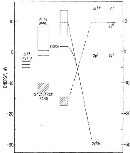
FIG. 2. Energy-level diagram for  $\text{Al}_2\text{O}_3$ . The displacement of the free-ion energy levels (shown at the right) when the lattice is formed is indicated by the dashed lines. The energy diagram as it seems to exist experimentally is shown to the left of center, and the approximate position of a typical  $3d$ -series ion (empty  $\text{Cr}^{2+}$  levels) relative to the band gap is shown at the left.
