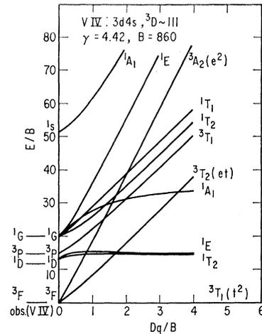
Fig. 1. Splitting of the free-ion energy levels of the electron configuration  $d^2$  due to a crystalline electric field having octahedral symmetry.  $E$  is the energy, and  $Dq$  and  $B$  are parameters that represent, respectively, the strength of the crystal field and Coulomb interaction between electrons (Ref. 6).
