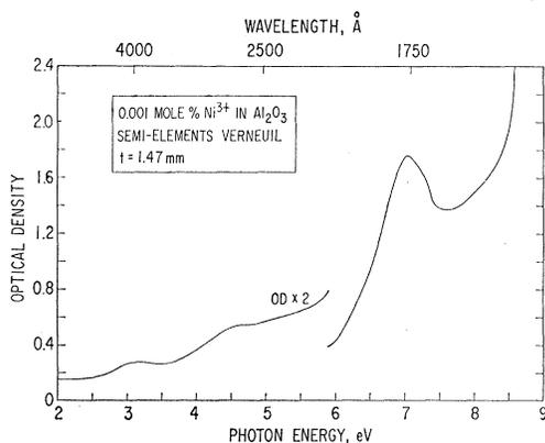
FIG. 10. Absorption spectrum of  $\text{Ni}^{3+}$  in  $\text{Al}_2\text{O}_3$ . The low-energy tail of the band peaked at 3.2 eV extends into the visible and gives the crystal a pronounced yellow color, even for very low Ni concentration.
