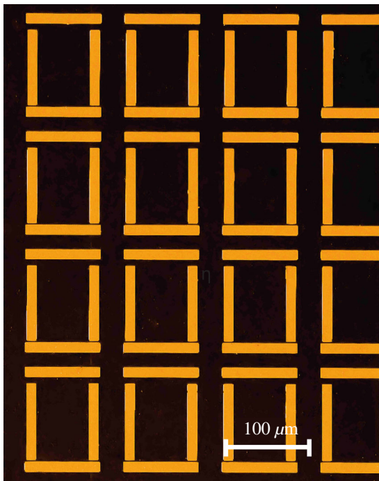
FIG. 7. SEM image of the fabricated rectangular ringlike structure.
