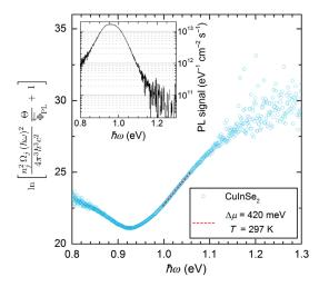
FIG. 2. Determination of  $\Delta\mu$  and  $k_BT$  from a linear fit in the high-energy range of the PL signal for a CuInSe<sub>2</sub> thin film deposited on a soda-lime glass substrate. The optical factor  $\Theta$  is determined from transmittance and reflectance measurements on the thin film plus substrate and on the bare substrate. (Inset) The corresponding PL spectrum for an emission in the  $2\pi$  sr in front of the sample.
