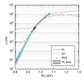
FIG. 3. Comparison of the absorption coefficient of a CuInSe<sub>2</sub> thin film deposited on soda-lime glass substrate measured by various methods (PL, photoluminescence; SP, spectrophotometry; PDS, photothermal deflection spectroscopy).
