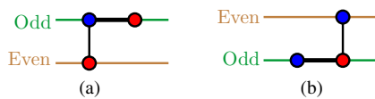
FIG. 8. The CZ gates between system (blue) and ancilla (red) qubits. (a) Right-closed hopping terms (between an odd-numbered row and the row below it), e.g., the one involving qubit 2 in Fig. 4(b). (b) Left-closed hopping terms (between an even-numbered row and the row below it), e.g., the one involving qubits 6 and 11 in Fig. 6(a).
