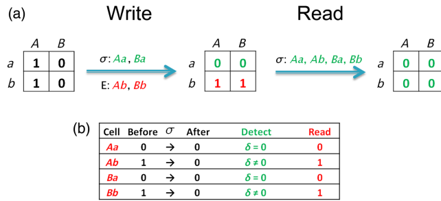
FIG. 7. Writing and reading bits processes. (a) Mechanically reversible domains are denoted as the logical signal 0 while mechanically irreversible domains are the logical signal 1. In the writing process, by applying the bias to cells Ab and Bb , and mechanical loading to cells Aa and Ba , the logical states of the 4 cells become Aa(0) , Ab(1) , Ba(0) , and Bb(1) , which are independent of their initial states. In the reading process, mechanical loading is applied to the cells and transfers logical states in the cells to the mechanically reversible state (0). (b) By detecting the change of the polarization \delta , cells are read 0 when \delta = 0 or 1 when \delta > 0 . Cells are therefore read Aa(0) , Ab(1) , Ba(0) , and Bb(1) .
