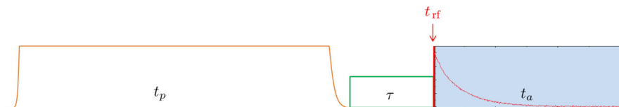
FIG. 4. By varying light duration t_p the polarization buildup rate can be measured, Fig. 8. By varying \tau , the time in the dark after the polarization is fully built up, relaxation rates which characterize the sensor can be determined, Fig. 9 and Table I. By varying the rf pulse strength, Fig. 3, the magnetic field can be calibrated. Details for buildup, vary- \tau , and ESR experiments can be found in Table III.
