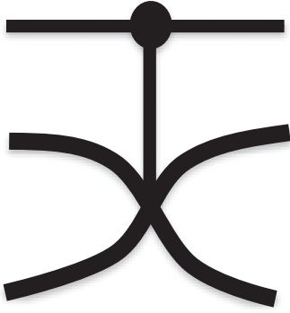
FIG. 3. The quantum-circuit representation of Fredkin (controlled-SWAP) gate. The horizontal solid back line is the circuit wire, the filled circle denotes the control qubit, and the large cross sign shows the SWAP gate which acts on the target qubits (the second and third qubits).
