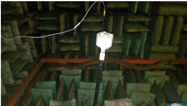
FIG. 8. Photo of the active metamaterial sensing device.
