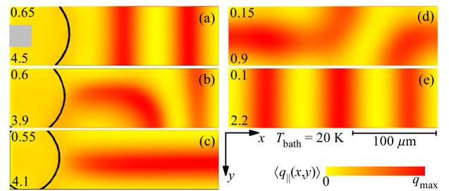
FIG. 2. Power density  $\langle q_{\parallel}(x, y) \rangle$  in units of  $10^{-5} \times j_{c0}^2 \rho_{c0}$  (color scale) for five values of normalized bias current  $I/I_{c0}$  (upper left numbers); values for  $q_{\text{max}}$  at the bottom left. The gray square in (a) indicates the position of the bond wire. Regions enclosed by the black line are at  $T_m \geq T_c$ .
