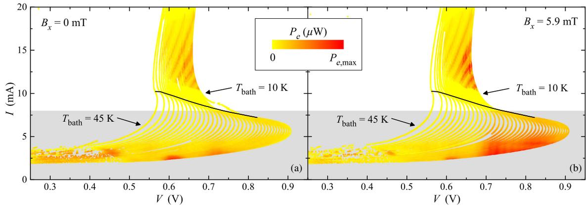
FIG. 4. Experimental data for a GBG structure: terahertz emission power  $P_e$  (color scale) for a large number of IVCs, measured at bath temperatures between 10 and 45 K for (a)  $B_x = 0$  and (b)  $B_x = 5.9$  mT. In both (a) and (b)  $P_{e,\max} = 27.5 \mu\text{W}$  for  $I > 8$  mA and  $P_{e,\max} = 0.21 \mu\text{W}$  for  $I < 8$  mA. Black lines in (a) and (b) indicate the  $T_c$  line.
