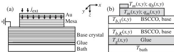
FIG. 1. Geometry used for modeling. Sketch of the mesa and electric current flow in the  $z$  direction (a). Geometry for thermal description (b), where  $q_m$  and  $q_b$ , respectively, denote the Joule power density produced in the mesa and by the bias lead. The temperatures of the various layers are indicated.
