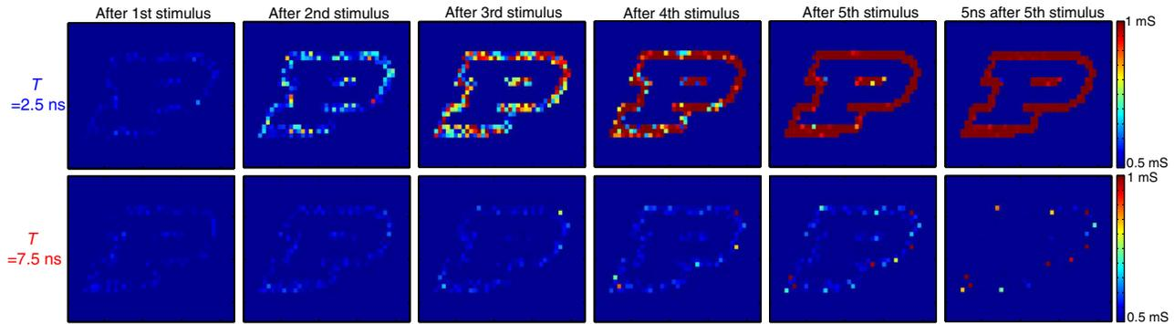
FIG. 5. STM and LTM transition exhibited in a  $34 \times 43$  MTJ memory array. The input stimulus is a binary image of the Purdue University logo, where a set of five pulses (each of magnitude  $100 \mu\text{A}$  and  $1 \text{ ns}$  in duration) is applied for each on pixel. While the array transitions to LTM progressively for frequent stimulations at an interval of  $T = 2.5 \text{ ns}$ , it “forgets” the input pattern for stimulation for a time interval of  $T = 7.5 \text{ ns}$ .
