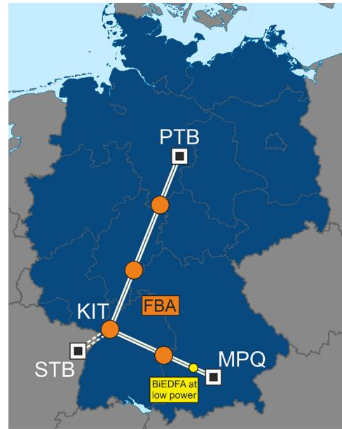
FIG. 1. The 940-km-long IFL between PTB and MPQ, shown on a map of Germany (in blue). Due to attenuation of the link laser light, four fiber Brillouin amplifiers (FBAs) [34] and one bidirectional erbium-doped fiber amplifier (BiEDFA) have been installed along its path. At Karlsruhe Institute of Technology (KIT), the IFL from PTB branches to MPQ and Strasbourg (STB).
