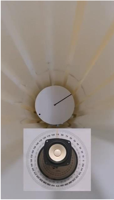
VIDEO 2. Counterclockwise rotation of the foam disk. This reveals the torque effect of an excited -1 order acoustic vortex. The vortex transfers the OAM from the wave to the foam disk, and then the foam disk rotates counterclockwise.
