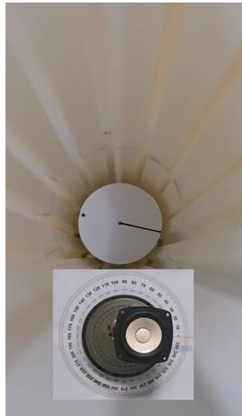
VIDEO 1. Clockwise rotation of the foam disk. This reveals the torque effect of an excited +1 order acoustic vortex. The vortex transfers the OAM from the wave to the foam disk, and then the foam disk rotates clockwise.
