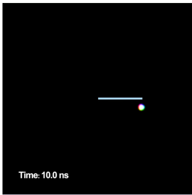
VIDEO 1. Motion of skyrmion ( \pi QP) when applying STT with a current density of 5.10^{11} A/m 2 (blue line is a reference line).
