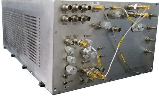
FIG. 7. Photograph of the atomic clock prototype, the size is 18 cm (height) \times 28 cm (width) \times 45 cm (length).
