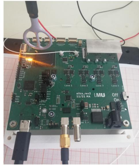
FIG. 8. Photograph of the measurement setup for the revised electronics. The USB-C connection (bottom left) acts as a power supply and the SMA connection (bottom center) supplies the trigger signal for time synchronization. The fiber-connected optics module (top right) was switched off during our measurements so as to test the electronics. When active, its dedicated metal casing effectively shields rf emissions.
