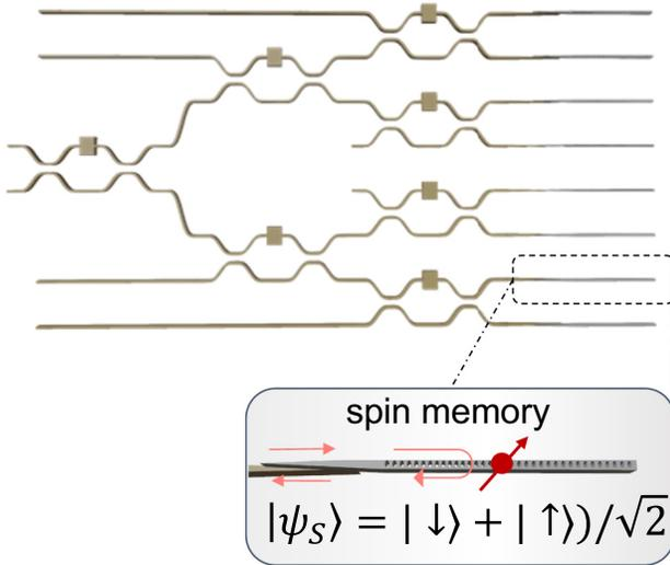
FIG. 13. Illustration of a MZI tree network as the interposer to the memories. Each layer introduces transmission loss from the MZI.
