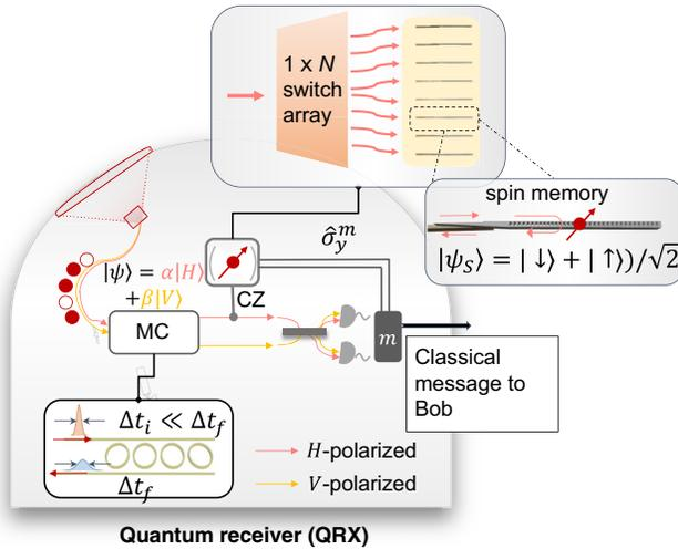
FIG. 4. Implementation of QRX—the QRX contains a MC and a  $1 \times N$  switching array that routes the photon to arbitrary channels in the memory bank, each containing a diamond nanocavity coupled with an optically active electron spin (red).
