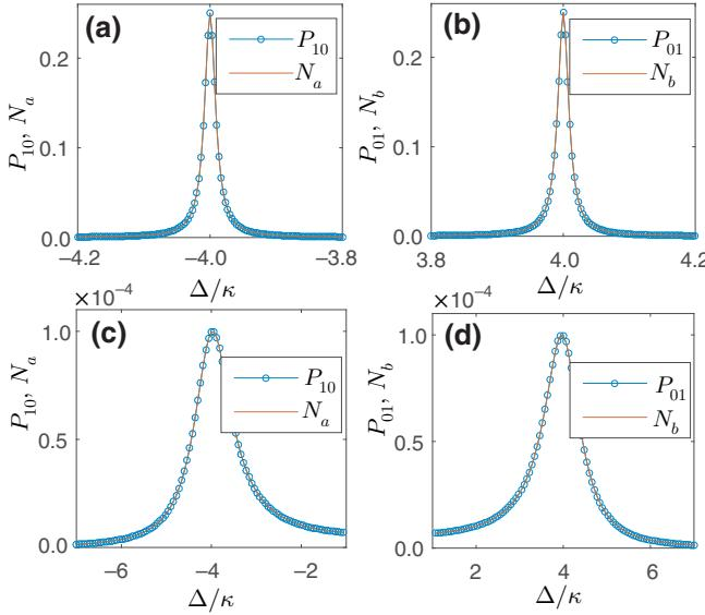
FIG. 4. Single-photon probability and average photon number as a function of the detuning  $\Delta/\kappa$  for EPB and CPB. (a) EPB for cavity  $a$ . (b) EPB for cavity  $b$ . In both (a),(b),  $g/\kappa = 4$  and  $\varepsilon/\kappa = 0.01$ . (c) CPB for cavity  $a$ . (d) CPB for cavity  $b$ . For both (c),(d),  $U/\kappa = 10$ ,  $J/\kappa = 4$ , and  $\varepsilon/\kappa = 0.01$ .
