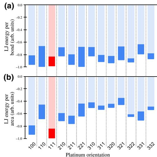
FIG. 2. The optimal Lennard-Jones energy (“goodness” of match) calculated between  $\beta$ -Ga<sub>2</sub>O<sub>3</sub> ( $\bar{2}01$ ) and all symmetry-inequivalent Pt planes with Miller indices between  $-3$  and  $3$  (a) per pair of matched Pt-O atoms (i.e., the Lennard-Jones “bond”) and (b) per unit area of the interface. The values are normalized to 1.
