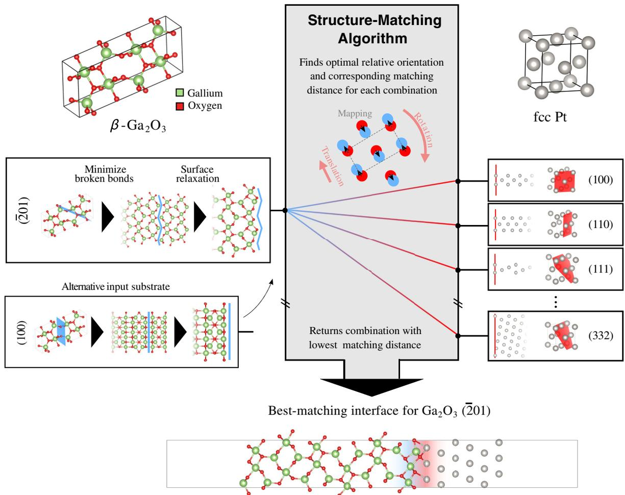
FIG. 1. The workflow to construct interfacial atomic structures. The structure-matching algorithm represented by the box in gray takes as an input a  $\beta\text{-Ga}_2\text{O}_3$  surface (left) and a set of Pt surfaces (right). It returns the interface structure of the best matching combination of interfaces.
