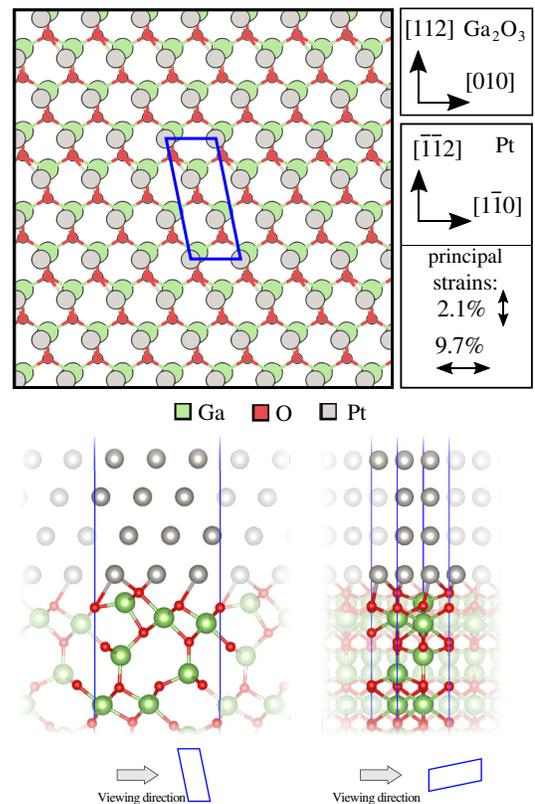
FIG. 3. The optimally matched interface structure between  $\beta$ -Ga<sub>2</sub>O<sub>3</sub> ( $\bar{2}01$ ) and Pt(111) corresponding to the red bars in Fig. 2. The in-plane periodic unit cell of the interface is represented by a blue parallelogram. Outward-pointing arrows indicate tensile strain. The strains apply to Pt only.
