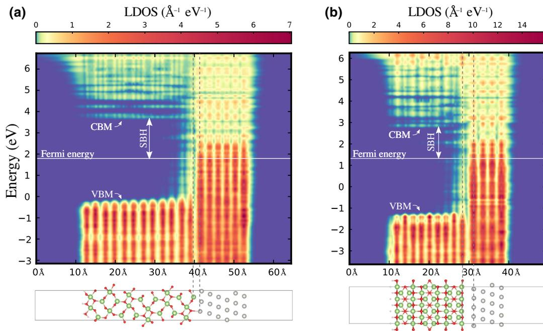
FIG. 4. The LDOS for (a) the  $\beta$ -Ga<sub>2</sub>O<sub>3</sub> ( $\bar{2}01$ ) and Pt(111) interface and (b) the  $\beta$ -Ga<sub>2</sub>O<sub>3</sub>(100) and Pt(111) interface. The Fermi energy is shown as a white line and the  $x$  axis is in line with the corresponding relaxed structure.
