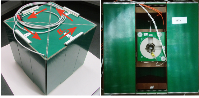
FIG. 2. Photographs of the field-confining coil used in this work. It is entirely made out of printed circuit boards (PCBs). On the left, the full coil is shown with \alpha , \beta , \gamma , and \delta quadrants, which open via nonmagnetic PCB headers (long white connectors). The arrows on the top panel show the direction of the magnetic field when applying a positive current. On the right, an open quadrant with the mount and a Cs magnetometer is shown. The fibers and cables used for the magnetometer leave the coil through a hole in the top. Temperature sensors (DS18B20; white spots in the mount) are glued into the mount on the top and bottom.
