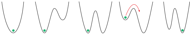
FIG. 5. Semiclassical picture of the dynamics. Left (right) corresponds to early (late) in the anneal. The green circle corresponds to the position of the system in the energy landscape.
