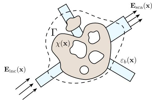
FIG. 1. A schematic showing an electromagnetic device within the region  $\Gamma$  with contrast  $\chi(\mathbf{x})$  embedded in an electromagnetic background with permittivity distribution  $\varepsilon_b(\mathbf{x})$ , excited with an incident electromagnetic field  $\mathbf{E}_{\text{inc}}(\mathbf{x})$  to produce a scattered field  $\mathbf{E}_{\text{sca}}(\mathbf{x})$ .
