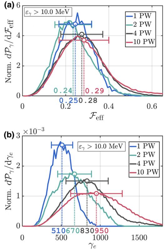
FIG. 5. Emitted power  $\mathcal{P}_\gamma$  for photons with  $\varepsilon_\gamma > 10$  MeV emitted into a single lobe as a function of (a)  $\mathcal{F}_{\text{eff}}$  and (b)  $\gamma_e$  at the time of peak emission (see Fig. 3) for  $P = 1$ –10 PW. The dashed lines show the average  $\mathcal{F}_{\text{eff}}$  and  $\gamma_e$ . The horizontal bars show the standard deviation. The area under each curve is normalized to be equal to unity.
