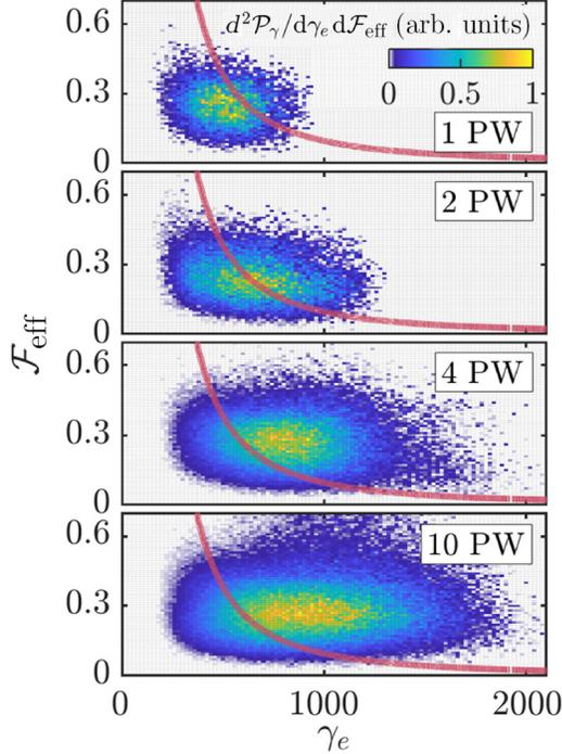
FIG. 4. Emitted power  $\mathcal{P}_\gamma$  as a function of  $\mathcal{F}_{\text{eff}}$  and  $\gamma_e$  at the time of peak emission (see Fig. 3) for  $P = 1$ –10 PW.  $\mathcal{P}_\gamma$  is for photons with  $\varepsilon_\gamma > 10$  MeV emitted into a single lobe. The curve corresponds to  $\varepsilon_\gamma^* = 10$  MeV [see Eq. (4)].
