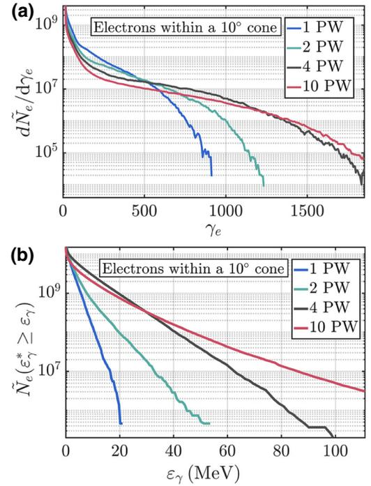
FIG. 6. (a) Normalized electron spectra at the moment of peak emission for  $P = 1$ –10 PW. (b) Accumulated number of electrons with  $\varepsilon_\gamma^* > \varepsilon_\gamma$ , defined by Eq. (8), as a function of  $\varepsilon_\gamma$ . Here  $\varepsilon_\gamma^* \approx 0.44\eta\gamma_e m_e c^2$  is the characteristic photon energy of a synchrotron spectrum. We count only the electrons whose momentum is directed within a single emission lobe.
