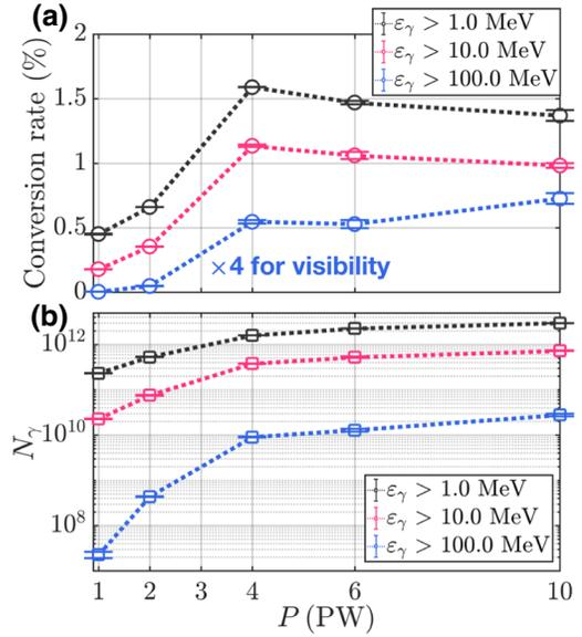
FIG. 2. Efficiency of conversion of laser energy into photons (a) and number of photons emitted into a  $10^\circ$  lobe (b) for different photon energies ( $\varepsilon_\gamma > 1, 10$ , and 100 MeV) as functions of the incident laser power  $P$  at a fixed peak intensity of  $5 \times 10^{22}$  W/cm<sup>2</sup>. Both the efficiency and the photon number are averaged over the right and left lobes, with the error bars giving the deviation from the average.
