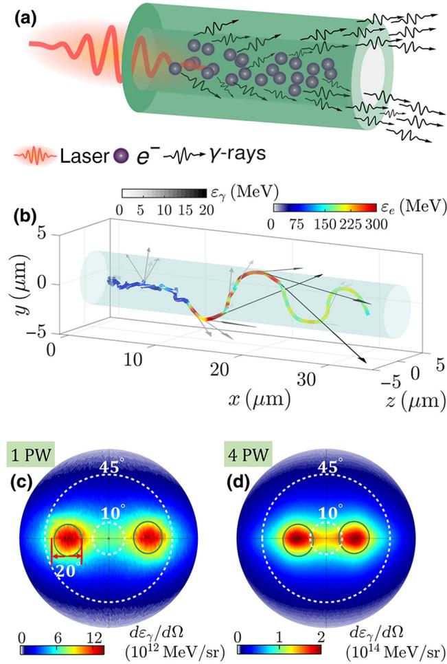
FIG. 1. (a) Schematic setup for generation of a directed  $\gamma$ -ray beam from a laser-irradiated structured target. (b) Representative electron trajectory, with the grayscale arrows showing the direction and energy of photon emission. (c),(d) Resulting  $\gamma$ -ray beams with  $\epsilon_\gamma > 1$  MeV at incident powers of 1 and 4 PW. The green circles show what we define as lobes.
