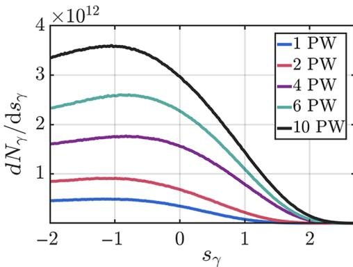
FIG. 10. Energy spectra of  $\gamma$ -ray beams generated with different laser powers. Here, “ $\gamma$ -ray beam” still refers to the photons emitted into a narrow cone with an opening angle of  $10^\circ$ . We use  $s_\gamma \equiv \log_{10}(\varepsilon_\gamma/\text{MeV})$  to cover a wide range of energies  $\varepsilon_\gamma$ .
