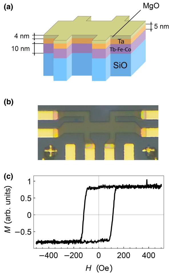
FIG. 1. (a) Scheme of structure with layers, (b) optical microscopy image of the Hall bar device. (c) Alternating gradient magnetometer measurement of magnetization loop of the film at room temperature.
