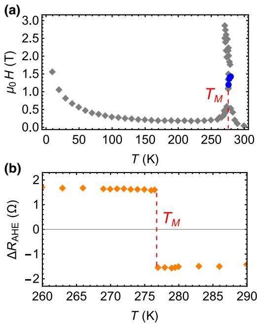
FIG. 3. Width, i.e., coercive field (a), and height,  $\Delta R_{\text{AHE}}$  (b), of the central hysteresis loop of the anomalous Hall effect as functions of temperature. The compensation temperature is  $T_M \approx 277$  K.
