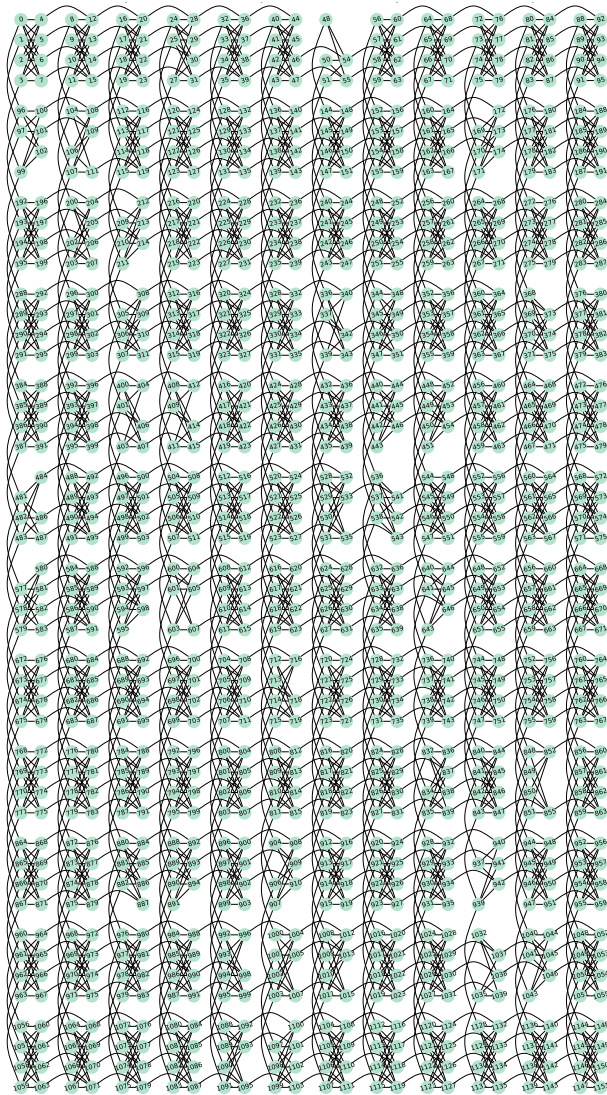
FIG. 7. Device architecture and qubit connectivity. The array of superconducting quantum bits is arranged in 12 \times 12 unit cells that consist of eight quantum bits each. Within a unit cell, each of the four qubits on the left-hand partition (LHP) connects to all four qubits on the right-hand partition (RHP), and vice versa. A qubit in the LHP (RHP) also connects to the corresponding qubit in the LHP (RHP) of the units cells above and below (to the left and right of) it. Edges between qubits represent couplers with programmable coupling strengths. We show only the 1097 functional qubits out of the 1152 qubit array.
