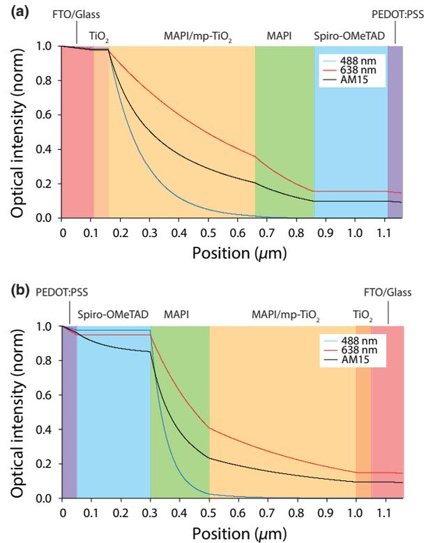
FIG. 9. Optical modeling of the mp- $\text{TiO}_2$  device with TCA electrode used in the transient photovoltage measurements. Optical intensity as a function of position for the mp- $\text{TiO}_2$  device stack incorporating the TCA electrode. Illumination from (a) the FTO-glass side and (b) the TCA side. Blue and red curves indicate wavelengths of 488 nm and 638 nm respectively, while the black curve shows the decay of the AM1.5 spectrum integrated from 300 to 768 nm.
