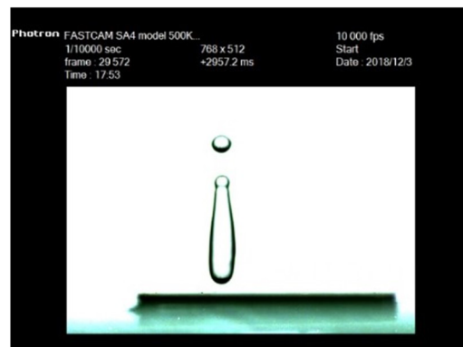
VIDEO 2. Droplet impact from height of a 5 cm for the 15-min sample.
