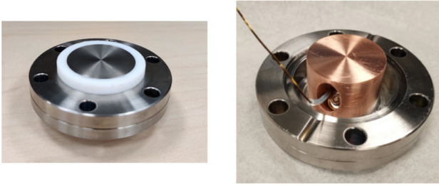
FIG. 4. A sample flange with the PTFE ring and Cernox sensor installed.
