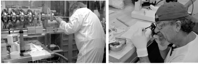
FIG. 58. Identifying particulate sources. Left: collecting particulates from a five-cell cavity previously operated with beam for reconstructing contamination distribution and offline determination of particulate sizes and compositions; right: inspecting the sealing surface of a beamline gate valve Viton seal aided with a magnifying glass for large particulates.
