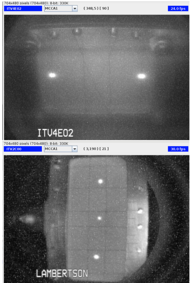
FIG. 35. Viewers showing 16.5 mm of separation in front of the second pass YA thin septum (above) and three beams at their proper elevation at the entrance to the Lambertson magnet for halls A, B, and C (below).
