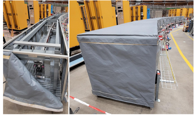
FIG. 26. Vacuum arc with its frame installed in the oven (left) is pumped with turbo-pump/primary pump stations during the heat up cycle (right).
