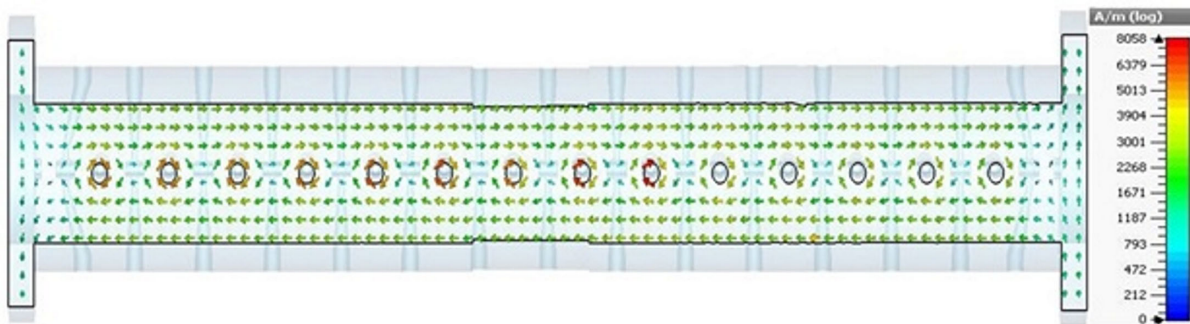
FIG. 12. Magnetic field distribution of the H_{210} mode in a horizontal plane above the beam axis as indicated in Fig. 18 by \overline{AA'} .
