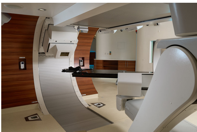
FIG. 3. Proton gantry treatment room with rolling floor, automatic robotic patient-positioning system with patient couch, and exit from the gantry nozzle. Gantry angle at 60° (0° gantry angle is defined as the upright gantry position with the output beam pointing vertically downward).
