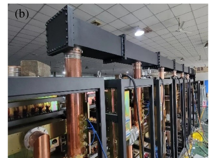
FIG. 14. (a) Principle of the chain combiner. (b) High-power experiment of chain combiner.
