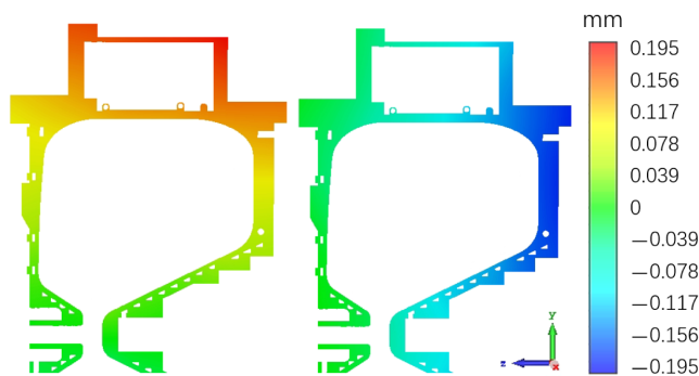
FIG. 10. Radial (left) and axial (right) deformation of the VHF gun due to thermal expansion.
