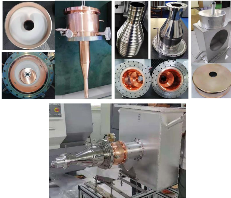
FIG. 20. FPCs' components and assemblies during the fabrication.
