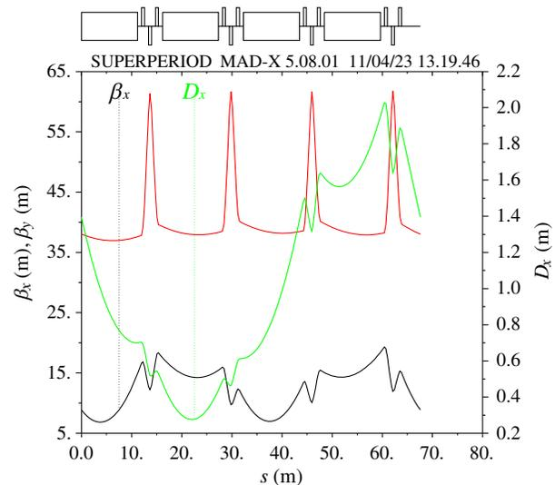
FIG. 5.  $\beta$  functions for horizontal and vertical planes and dispersion in the horizontal plane are shown for one superperiod of the new AGS lattice. In this case, it is optimized using Eq. (8).
