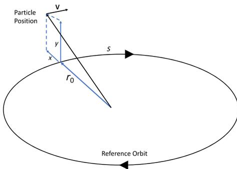
FIG. 1. The curvilinear coordinate system for particle motion in a circular accelerator. The unit vectors  $\hat{x}$ ,  $\hat{s}$ , and  $\hat{y}$  are the transverse radial, longitudinal, and transverse vertical basis vectors; and  $\vec{r}_0(s)$  is the reference orbit.
