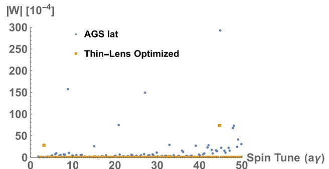
FIG. 6. DEPOL calculated spin resonances for the proton AGS machine and the toy AGS-like machine with periodicity of 12 and spin cell suppression.
