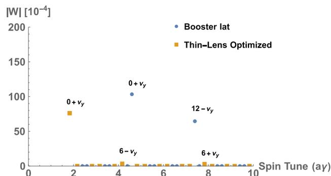
FIG. 2. DEPOL calculated spin resonances using vertical emittance of 10 mm mrad with the lattice employing the special intrinsic spin resonance suppressing cell. This is compared to a standard FODO cell with dipoles in-between BNL's booster lattice. Here the strongest intrinsic spin resonances are labeled.
