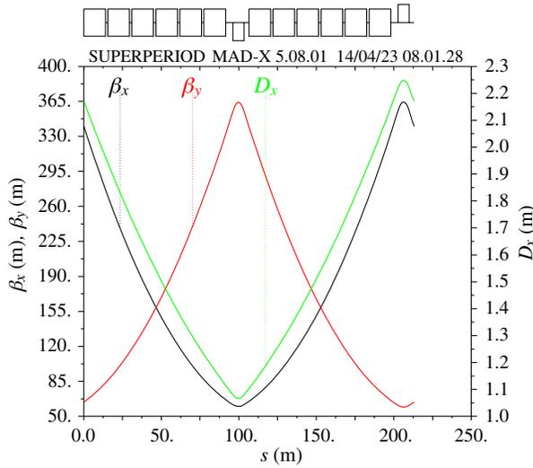
FIG. 7.  $\beta$  functions for horizontal and vertical planes and dispersion in the horizontal plane are shown for one FODO cell of the arc FCC-h lattice (per 2019 CDR).
