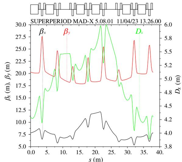
FIG. 4.  $\beta$  functions for horizontal and vertical planes and dispersion in the horizontal plane are shown for one superperiod of the new booster lattice. In this case, it is optimized using Eq. (8).
