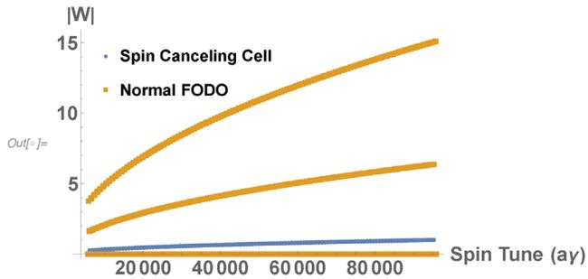
FIG. 9. DEPOL calculated spin resonances for a FCC-hh arc only (no insertions) lattice using standard FODO cell construction versus an FCC-hh like lattice with three quad arc cells which suppress the spin resonances.
