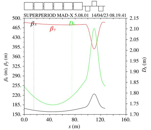
FIG. 8.  $\beta$  functions for horizontal and vertical planes and dispersion in the horizontal plane are shown for one dipole (similar to half standard FODO cell) of my Toy arc only FCC-h lattice.
