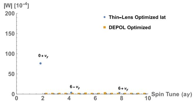
FIG. 3. DEPOL calculated spin resonances using normalized emittance of 10 mm mrad. Here we use the special intrinsic spin resonance suppressing cell for the booster. Here the thin-lens optimized optics using Eq. (8) and optics optimization using the DEPOL algorithm are compared. The strongest intrinsic spin resonances are labeled.
