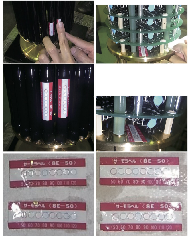
FIG. 33. The upper-left and upper-right panels show the cases where temperature labels are attached to the resistors and the metal plate below the diode part prior to 24-h operation of the kicker. The middle-left and middle-right panels show the resistors and metal plate after the operation. The lower-left and lower-right panels show the temperature labels detached from the resistors and the plate after the operation.
