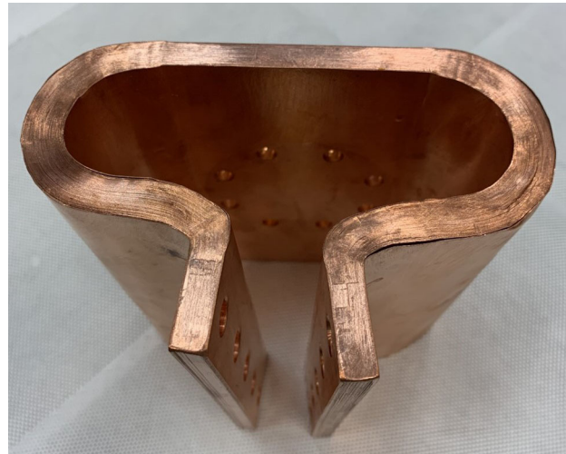
FIG. 17. Picture of the TLA used to connect the cavity to stage 2 of the CCR.
