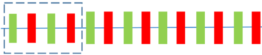
FIG. 4. Schematic plot of a FODO lattice used in the second application example. The four quadrupoles inside the dashed line box were used to match the initial distribution to the periodic FODO lattice.
