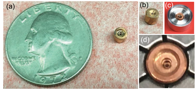
FIG. 7. Photos of the fabricated gun structures. (a) Cells with the coupling opening pointed up. The coupling iris and inner iris are both visible. (b) Back of the structure showing a divot for centering and alignment in the final assembly. (c) Cell structure upright in an aluminum adapter for cold testing. (d) Close-up photo where inner features are visible. The copper tip is visible in the center and the inner iris is also visible.
