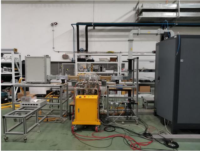
FIG. 13. The layout of rf test system for 1.3 GHz FPCs.
