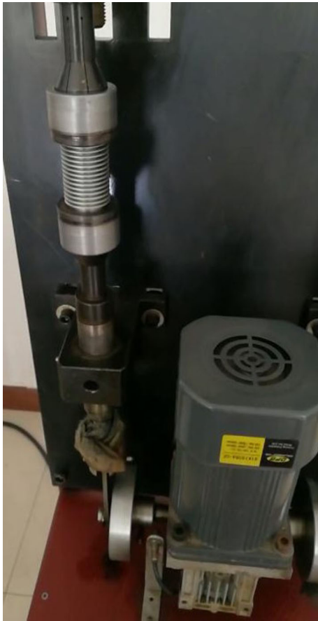
FIG. 10. Fatigue test of a 1.3 GHz coupler bellow.
