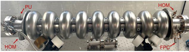
FIG. 1. Photo of TESLA shape nine-cell 1.3 GHz cavity, with highlighted ports for the higher order modes (HOM) couplers, the fundamental power coupler (FPC), and the pickup (PU) coupler.
