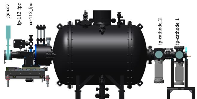
FIG. 3. Detailed view of the SRF gun cryostat with the critical vacuum components. The cathode insertion is on the right side of the schematic and the FPC is on the left side. Here ip = ion pump; tc = thermal conductivity gauge, reads pressure from atmosphere to  $1 \times 10^{-3}$  Torr; cc = cold cathode gauge, reads  $1 \times 10^{-3}$  to  $1 \times 10^{-11}$  Torr; sv = vacuum valve.
