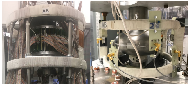
FIG. 6. Single cell cavity setup for evaluating sporadic quenching with a temperature map (left) and second sound sensors (right).
