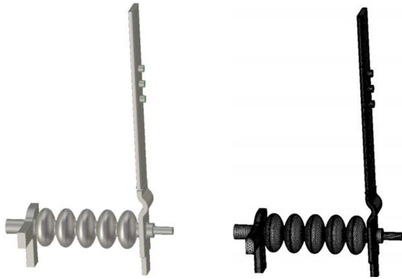
FIG. 18. The rf model (left) and mesh representation (right) for simulating a C50 cavity in a CM configuration.
