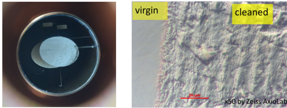
FIG. 7. Photograph of Mg photocathode Mg#214 after second laser cleaning (left) and surface structure changes after cleaning (optical microscope image, right).
