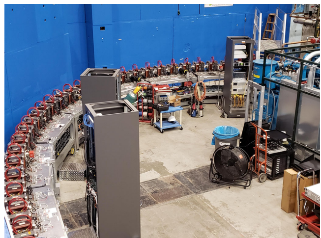
FIG. 3. Second arc of the installed CBETA return loop.
