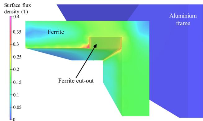
FIG. 7. Initial design of end ferrites, with cut-out to bend the saddle coils toward the aluminium frame (quarter of geometry shown). The color regions associated with the ferrite represent surface contours of predicted flux density, for a coil current of 240 A.
