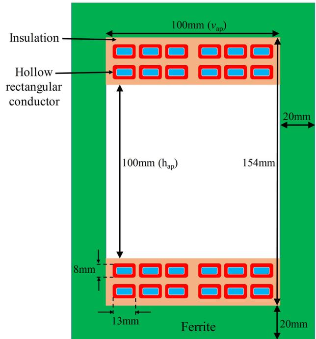
FIG. 6. Cross section of aperture of kicker magnet: rectangular coil conductors with 2 mm wall (red), insulation (brown), ferrite (green), and  $100\text{ mm} \times 100\text{ mm}$  aperture (white).
