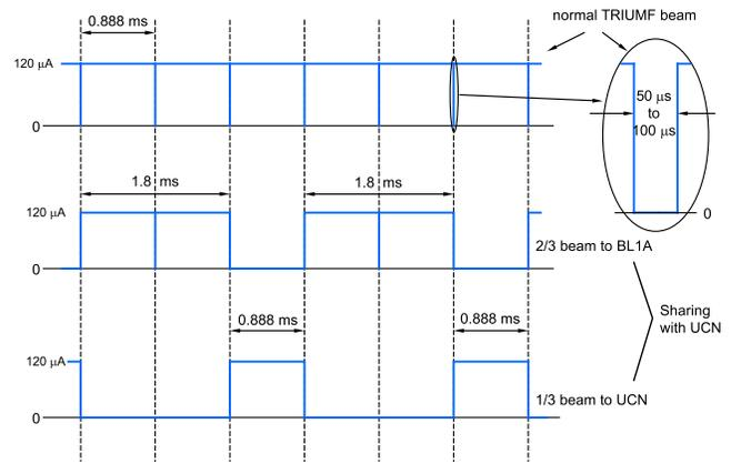
FIG. 1. Sharing of the main beam from the cyclotron (normal TRIUMF beam) between beamline 1A and beamline 1U. Beam is diverted into beamline 1U by switching on the kicker magnet during the 50–100  $\mu\text{s}$  notch duration, then switching it off during the next notch. The pulser period is 0.888 ms.
