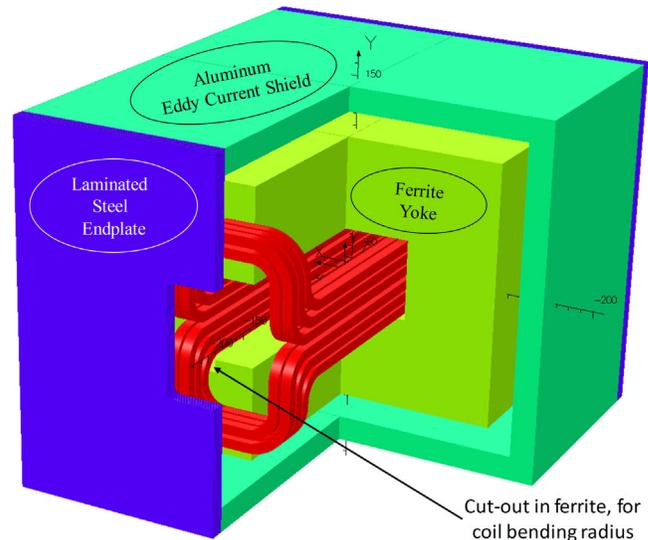
FIG. 3. Geometry of MedAustron kicker magnet, which served as a reference design for the TRIUMF kicker magnet. The overall length of the MedAustron magnet, including end plates, is  $\sim 0.4$  m.
