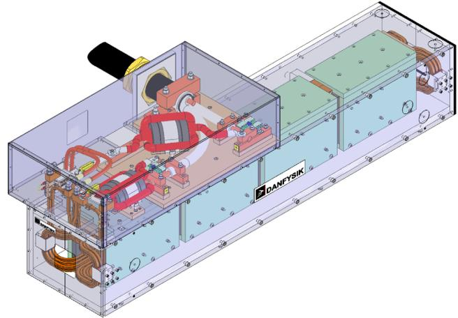
FIG. 9. 3D engineering drawing of the UCN kicker magnet and connection box. The overall length of the magnet is  $\sim 1.71$  m.
