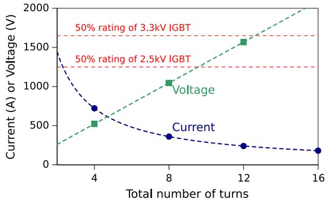
FIG. 4. Plot of the required magnet current and estimated magnet voltage to achieve a magnetic field integral of  $0.0545 \text{ T} \cdot \text{m}$ , as a function of the total number of turns of the magnet coils with a 1.5 m long yoke. End effects are neglected and  $h(\text{eff})_{\text{ap}} \times v_{\text{ap}} = 120 \text{ mm} \times 100 \text{ mm}$  is assumed.
