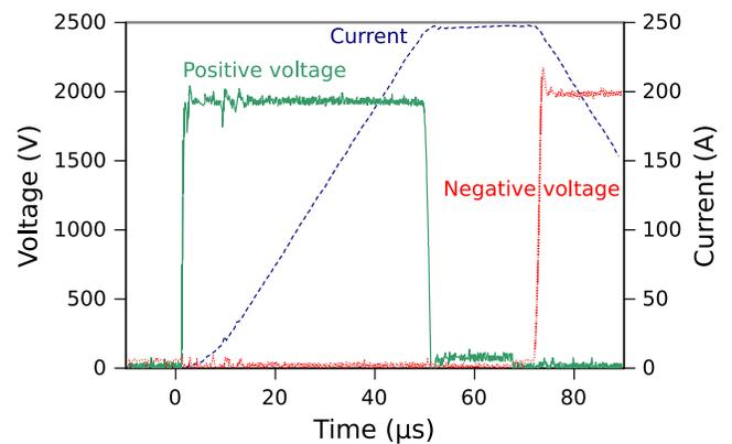
FIG. 12. Measured power-supply waveforms for 250 A demanded flat-top current, with 30 m of cable: Positive-side output voltage (green solid trace); negative-side output voltage (red dotted trace); output current (blue dashed trace).
