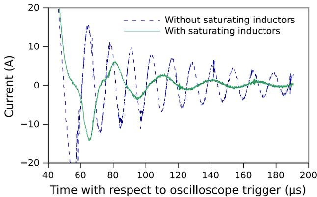
FIG. 10. Measured postpulse current following 250 A flat-top magnet current: without saturating inductors (blue dashed trace) and with saturating inductors (green solid trace).
