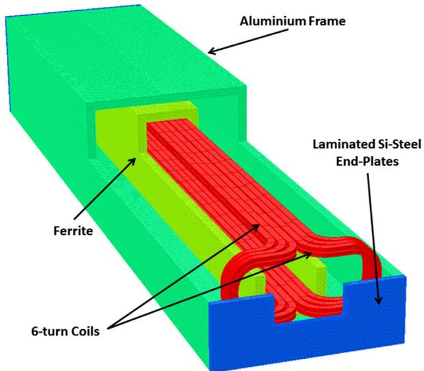
FIG. 5. Geometry for a 3D simulation of the UCN kicker magnet. The overall length of the magnet, including end plates, is  $\sim 1.71$  m.
