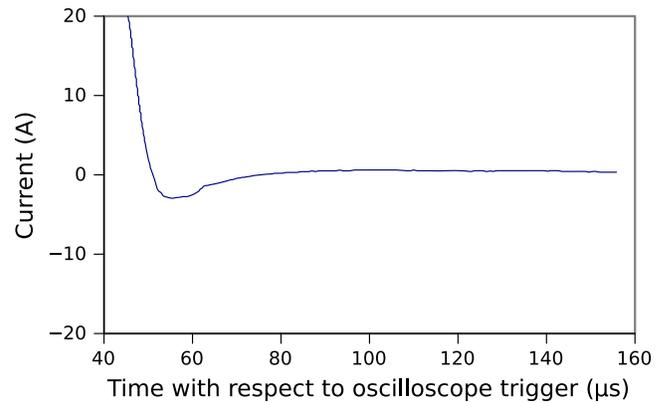
FIG. 11. Measured postpulse current following 250 A flat-top magnet current, without saturating inductors but with SF5408 fast recovery diodes, in a series/parallel arrangement, connected in series with diode D2.
