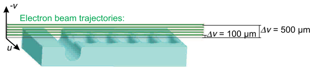
FIG. 5. Vertical relative position of the beam with respect to one half of the structure.
